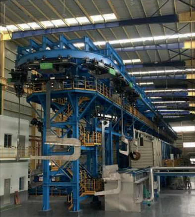
*Fully automatic ring track tunnel pickling and coating system for C-steel bundles with a ZLD*
