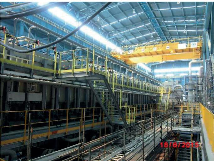
*Vertical roll-through pickling system for stainless steel, nickel and titanium plates*
